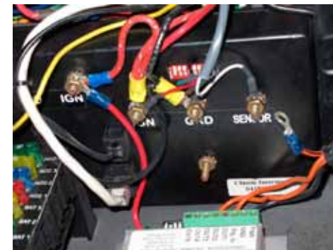
The disconnected wire you see (right) is the original speed hot wire. Note the white (sensor), red (ignition), and black (ground) are now installed.
