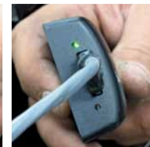
The "green" light means your Sky Drive has picked up the satellite signal and your speedo/odometer is ready to go.
