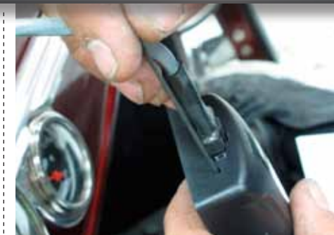
There is a pinhole that houses the calibration switch. We used a very small Allen wrench but a ballpoint pen or a paperclip will work as well.
