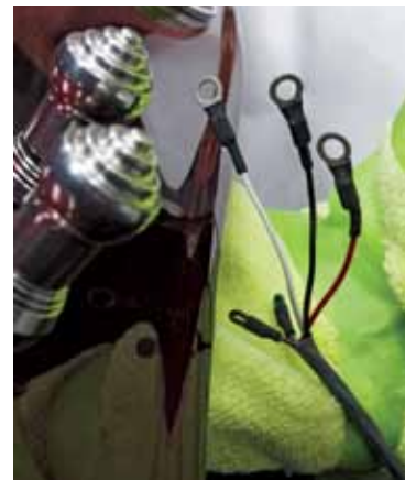
Since I only needed the basic installation I used the white (speed signal output), red (constant battery power), and black (chassis ground).
