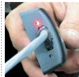
The "red" light means you have power and are ready to begin the calibration.
