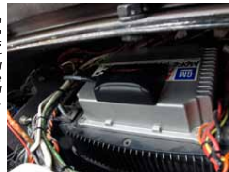
The disconnected wire you see (right) is the original speed hot wire. Note the white (sensor), red (ignition), and black (ground) are now installed.
