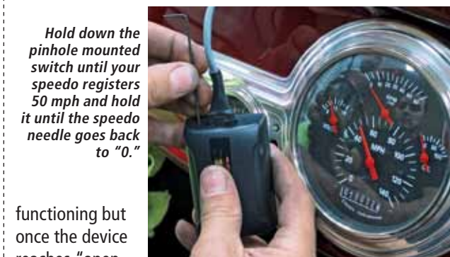
There is a pinhole that houses the calibration switch. We used a very small Allen wrench but a ballpoint pen or a paperclip will work as well.
