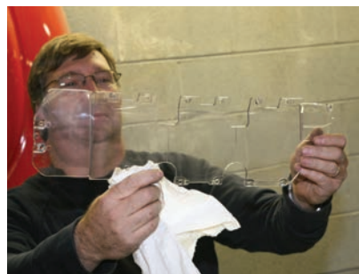
11. Before installing the lens on the new gauges, we made sure it was spotless and free of any dust or fingerprints.
