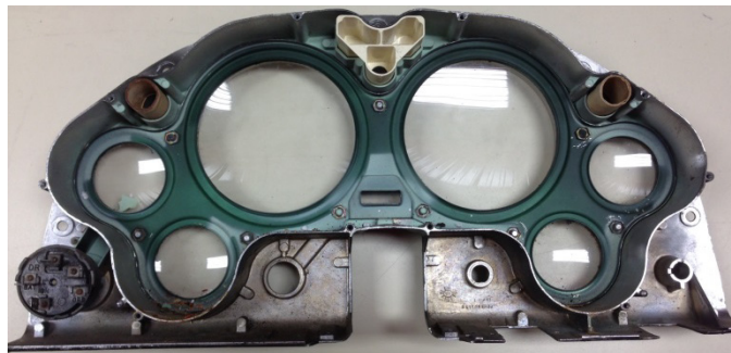
OEM Housing with Lenses & Holder
