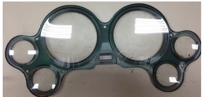
OEM Lenses and Holder Removed
