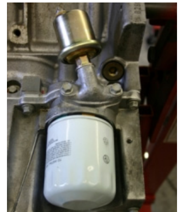
LS1 Oil Bypass Housing
