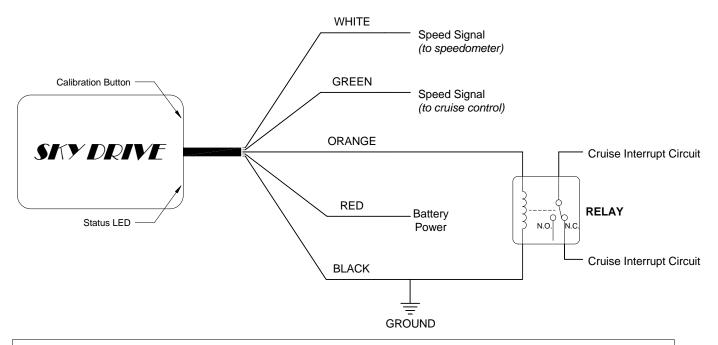
As a safety feature, the Sky Drive is designed to turn off the vehicle's cruise control in the event of a lost GPS signal. A two-second, 12-volt pulse is provided on the orange wire to drive a relay coil, which must be wired into the vehicle's cruise control interrupt circuit.
