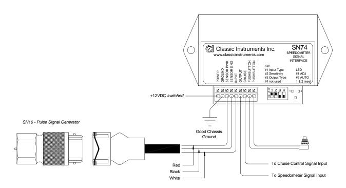
Module Connected to SN16 Pulse Signal Generator
