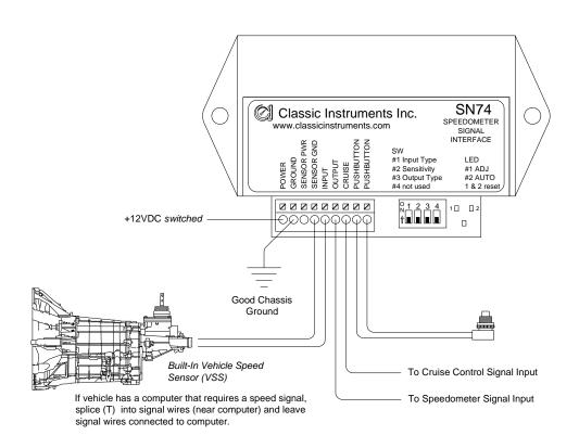
**Module Connected to Electronic Transmission's VSS**
