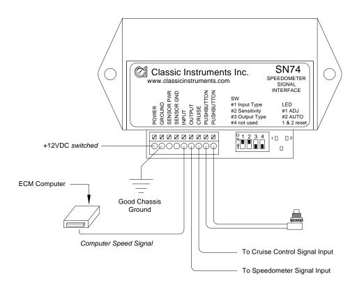
**Module Connected to ECM Speed Signal**
