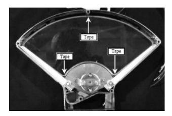
6) Place the gear selector gauge over the gear selector bracket.
