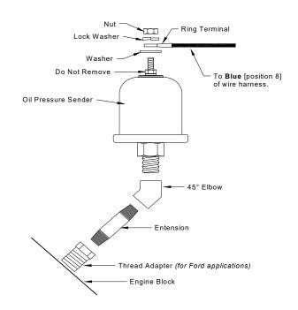
**GM Installation**: The correct location on most GM V8-engines to install the oil pressure sender is under the distributor housing at the rear of the block.
