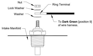
This is a copper based anti-seize which will allow a good electrical connection for the sender ground.
