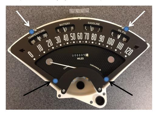
• Place new gauge cluster into the gauge bezel and secure using the 6 screws.
