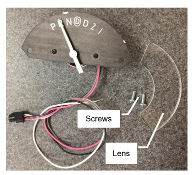
Remove the pointer from the original mechanical gear indicator assembly.
